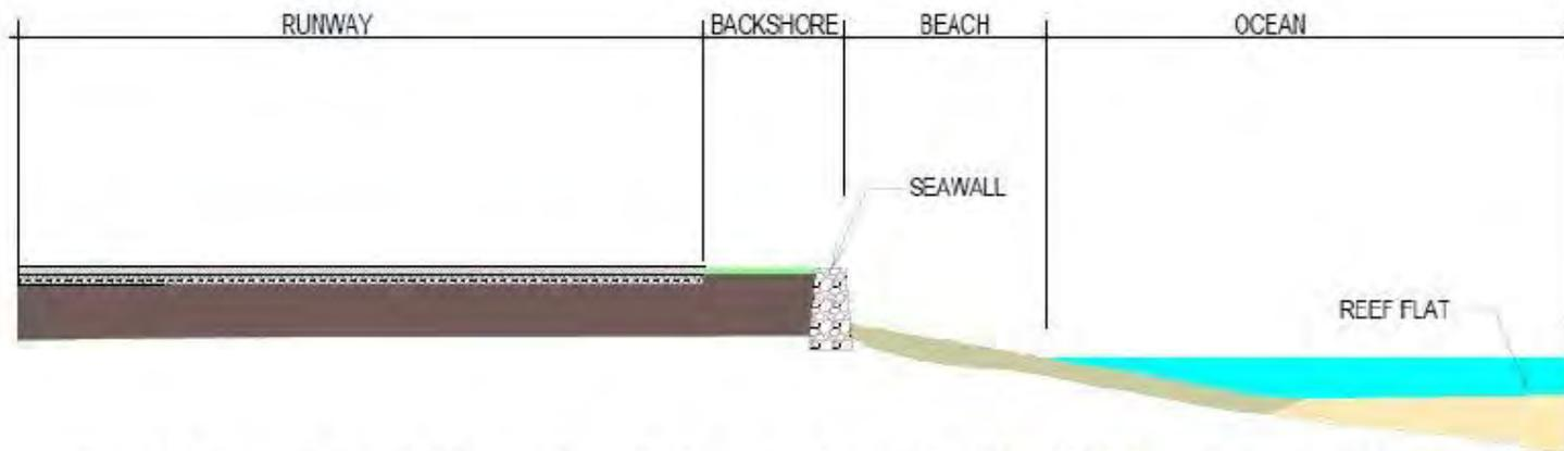
Figure 6: Concrete Rubble Masonry Seawall Alternative. Schematic of the CRM Seawall alternative design. Schematic provided by Corps.
