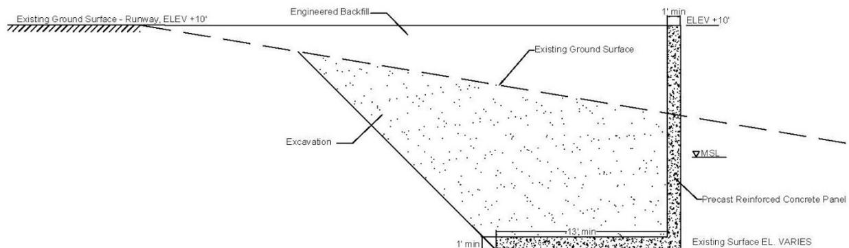
**Figure 22. Alternative 5 - Preliminary Precast Concrete Panel Wall Cross Section**
