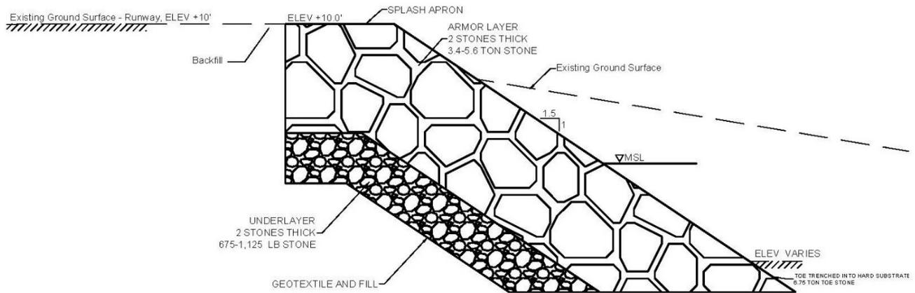
Figure 11: Alternative 1- Rock Revetment
