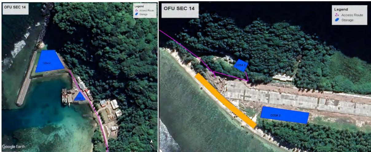
Figure 5. Staging Areas: COSA 3 and 4 at Ofu Harbor on the left and COSA 1 and 2 at Ofu Airport on the right. The tribar revetment structure is depicted in orange.
