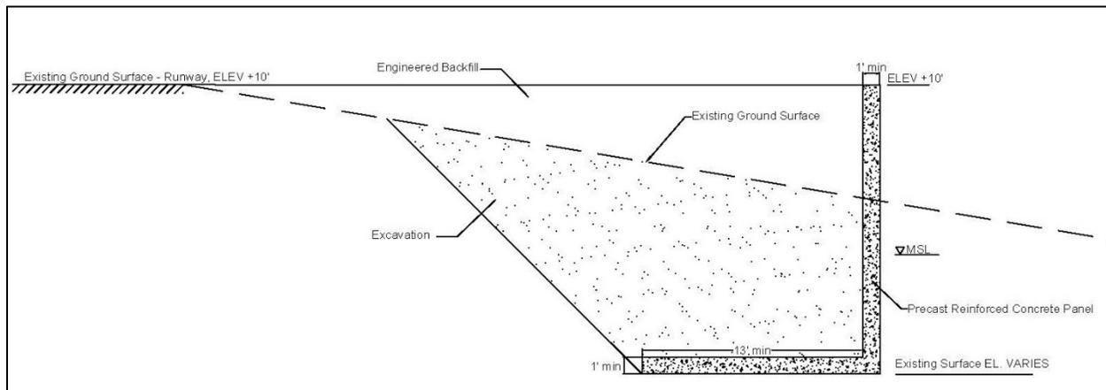
Figure 4 : Alternative 5 - Precast Concrete Seawall
