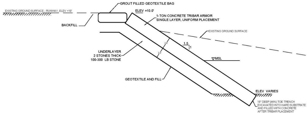
**Figure 20: Alternative 2 - Preliminary Tribar Concrete Armor Revetment Cross Section**
