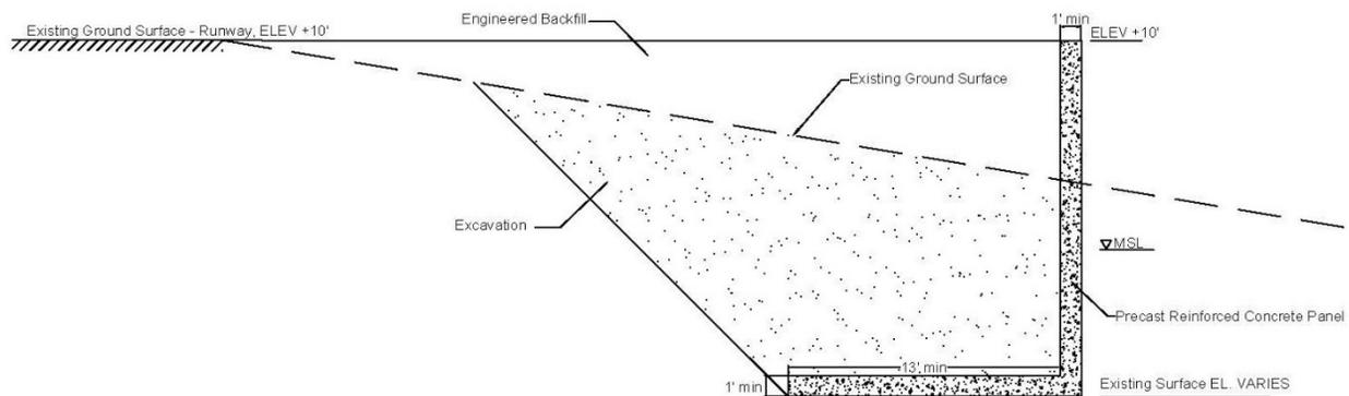
Figure 14: Alternative 5 - Precast Concrete Seawall
