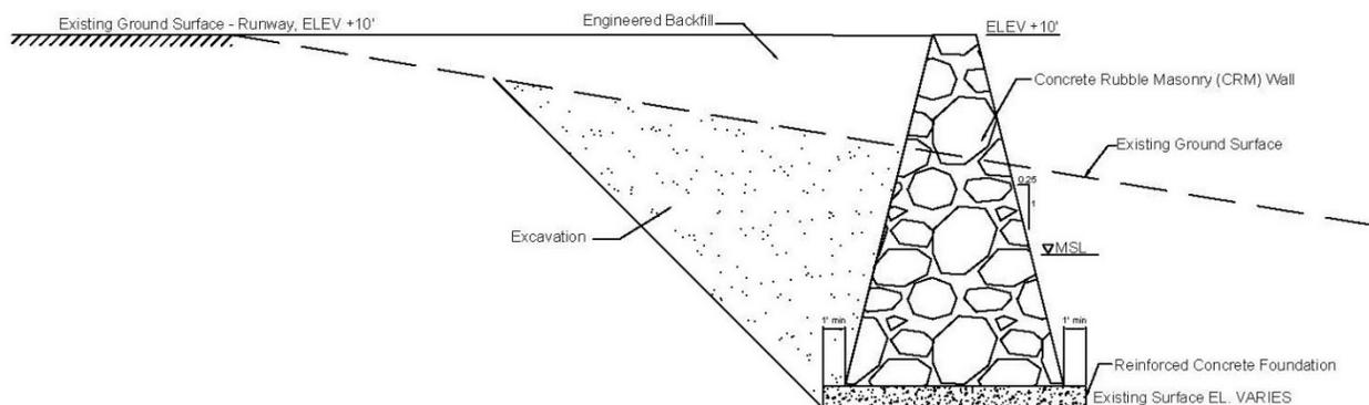
Figure 21. Alternative 3 - Preliminary CRM Wall Cross Section
