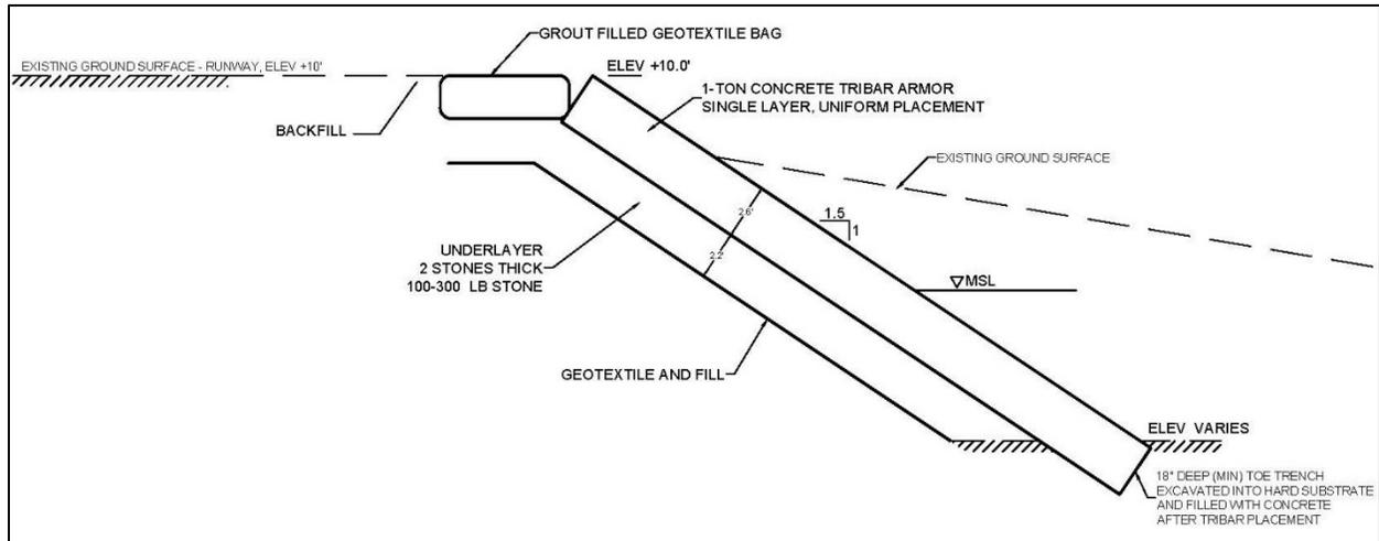
Figure 3: Alternative 2 – Tribar Revetment
