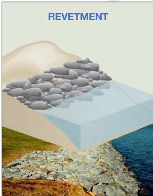
Figure 16. Revetment measure.
