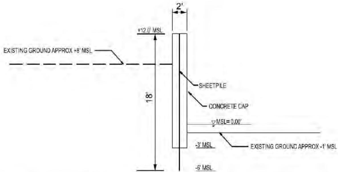
Figure 7: Sheetpile Seawall Alternative. Schematic of the Sheetpile Seawall alternative design. Schematic provided by Corps.
