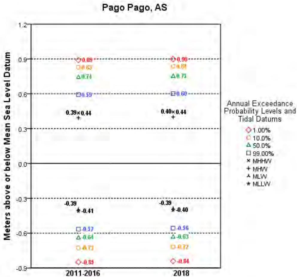
**Figure 9. AEP Water Levels relative to MSL**
