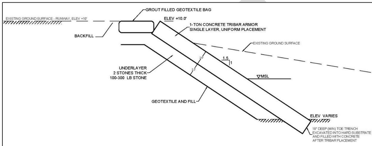
**Figure 1.** Alternative 2 – Tribar Revetment
