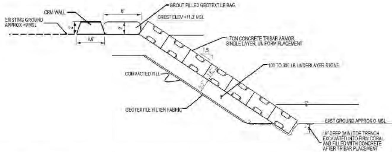
Figure 10: Tribar Revetment Alternative. Schematic of the tribar revetment alternative design. Schematic provided by Corps.
