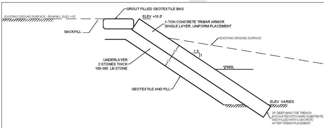
Figure 8. Preliminary Tribar Revetment Detail
