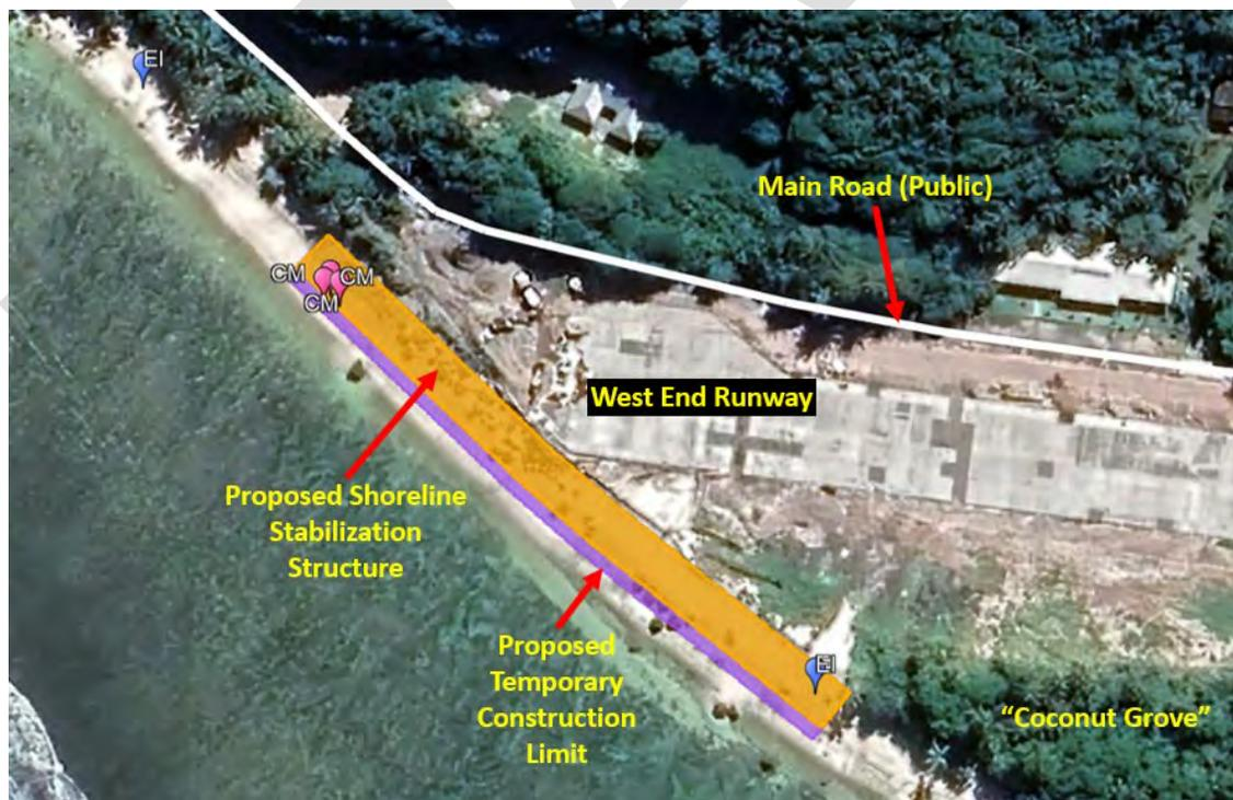
Figure 5. Project Feature Map. The orange shaded is the 0.38-acre tribar revetment (shoreline structure) to be constructed at the west end of the airport runway and the purple shaded area in
