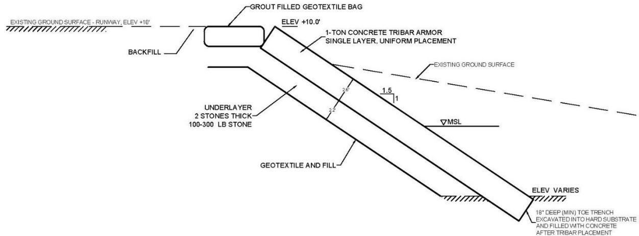
Figure 12: Alternative 2 - Tribar Revetment
