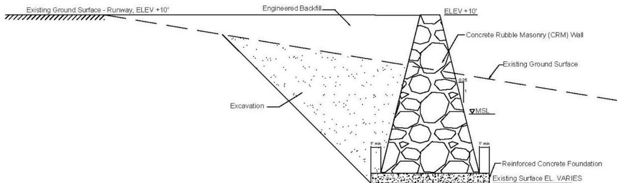
Figure 10. Preliminary CRM Seawall Cross Section Detail
