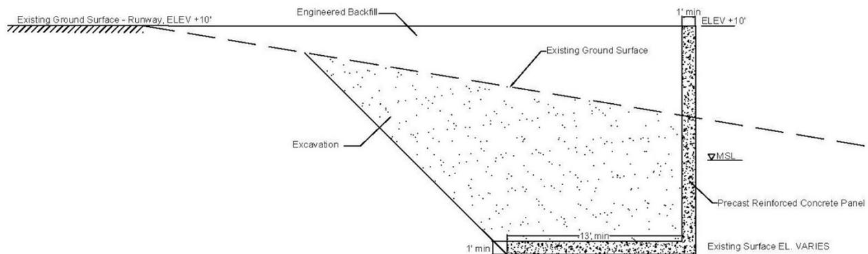
Figure 12. Preliminary Precast Concrete Seawall Detail
