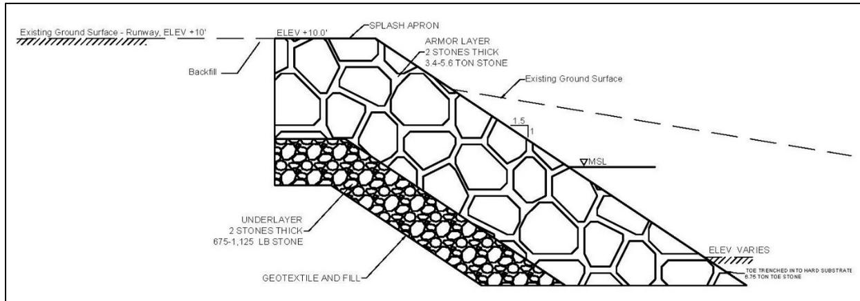
Figure 1: Alternative 1 - Rock Revetment
