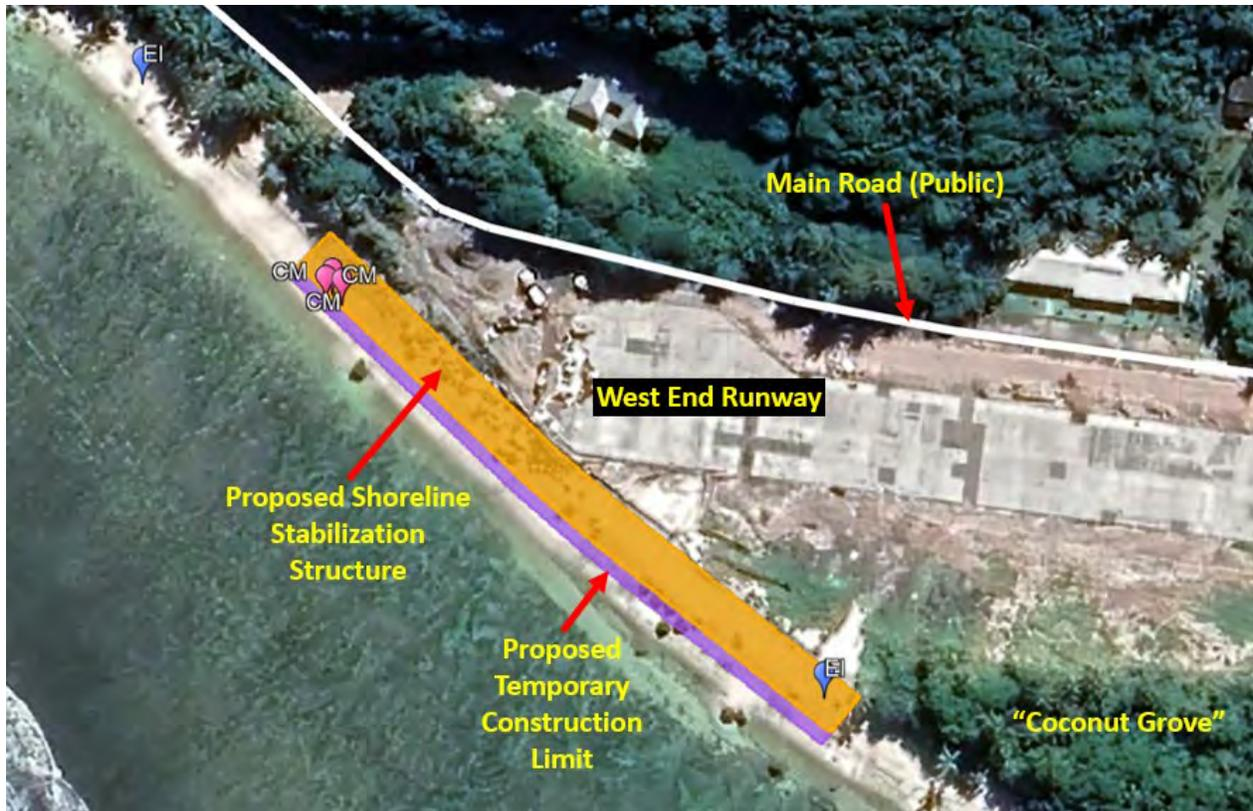
**Figure 5.** General location and placement of proposed Alternative 2: Tribar Revetment in relation to landscape features: Permanent Tribar Revetment (orange), temporary toe excavation (purple), and hawksbill (blue teardrop; EI) and green sea turtle (pink teardrops; CM) nests observed in 2017-2019 surveys by DMWR.
