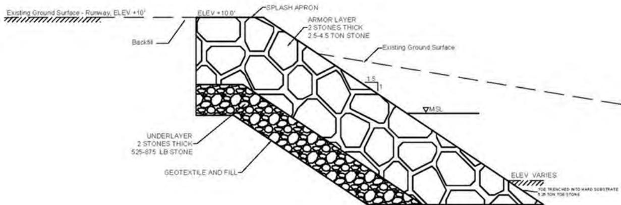
Figure 6. Preliminary Rock Revetment Detail
