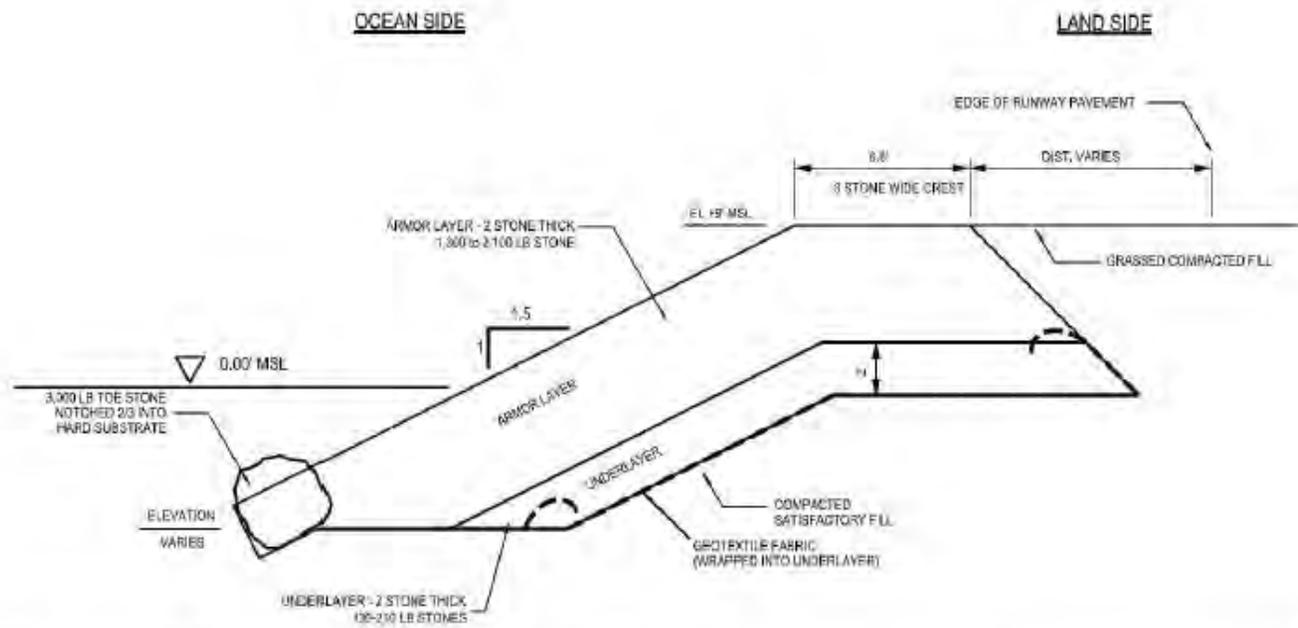
Figure 9: Rock Revetment Alternative. Schematic of the rock revetment alternative design. Schematic provided by Corps.
